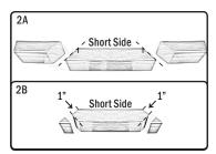
STEP #2A - Cut 45° miter on each end at the mark made in Step 1.
