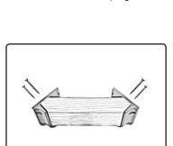
STEP #3 - Use 2 each screws to attach railing connector to 2x4. (Pre-drill holes if desired)
