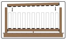
STEP #4 - With bottom rail mounted in place, insert all balusters into bottom rail. Start top rail at one end and insert connectors onto balusters. Make sure balusters are fully seated.
