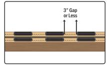
STEP #2 - Align top and bottom rails side by side. Lightly mark center line of 2x4. Determine number of glass balusters and layout glass baluster connectors evenly. Ensure the gap between connectors is no more than 3".
