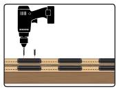
STEP #3 - After connectors are laid out correctly, use 2 each screws to fasten connector to rail.
