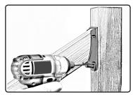
STEP #4 - Locate 2x4 railing on post and use 4 each screws to attach railing to post.
