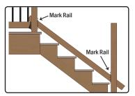
STEP #1 - Lay bottom 2x4 rail alongside posts and mark for angle. If posts are plumb top rail will be the same length and angle. Subtract 1/2" from overall length to account for 1/4" railing connector thickness. Cut 2x4s to create top and bottom stair rails.
