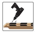
STEP #3 - After connectors are laid out correctly, use 2 each screws to fasten connector to rail.
