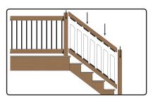
STEP #4 - With bottom rail mounted in place, insert all balusters into bottom rail. Start top rail at one end and insert connectors onto balusters. Make sure balusters are fully seated.
