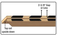
STEP#2 - Align top and bottom rails side by side with the top rail turned upside down as shown.
