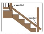
STEP #1 - Lay bottom 2x4 rail alongside posts and mark for angle. If posts are plumb top rail will be the same length and angle. Cut 2x4s to create top and bottom stair rails.
