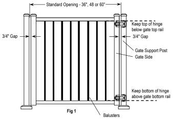
Follow installation instructions included with hinges and latches. NOTE: Align gate rails with adjacent railing when attaching gate to gate support post.
