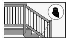
**Step 7:** Stair rails and balusters can present an installation challenge. Deckorators angled stair rail connectors (sold separately) create a snug and accurate baluster fit for stair angles at 35 degrees. Cut top and bottom stair rails at the proper angle. Lay top and bottom 2x4 rails alongside the posts and mark.
