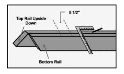
**Step 8:** Clamp the top and bottom rails together with the top 2x4 rail inverted. Position rails as shown and mark 5-1/2" on-center, working from the center out to the ends of the rails.
