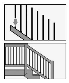
**Step 10:** Make sure connectors are properly aligned, apply silicone caulk to each stair connector, and assemble the top and bottom rails with the balusters. Then attach full rail section between the stair rail posts.
