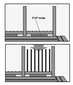
**Step 4:** Place the bottom rail between the rail posts, supported by a 3" block (2x4 scrap material works best). Secure rail to posts using Deckorators rail connectors (sold separately) and slide balusters over the bottom connectors. Carefully place top rail over the balusters, making sure each baluster is seated properly on each connector.
