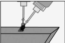
**Step 9:** Properly position the connectors on the rails. The top and bottom connectors will be facing opposite directions. Screw the connectors in place. To properly set angled connectors, begin screwing vertically until the screw bites into the wood. Reposition screw to the proper angle and tighten. Do not over-tighten, which can move the connector off center.
