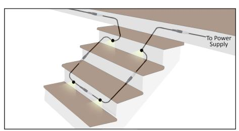
Step 4 - Wiring diagram
