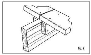
Pre-drill and countersink all deck screws, regardless of type, that are within 1-1/2" of the end of the deck board.
