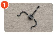
You will need 4 clips for each butt joint. Remove the legs of the EDGE Clips so that they can sit side-by-side on the double joists.
