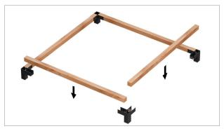
Place beams into connector slots as shown.
