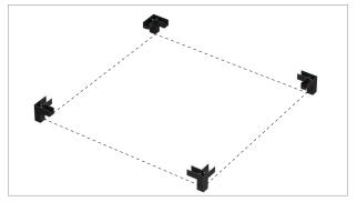
Arrange corner connectors into a square. To avoid scratching finish, set parts on cardboard or other soft material.
