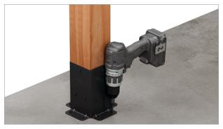
Predrill holes for anchors using a 3/16" concrete drill bit. Install provided screw anchors to secure pergola to concrete.
