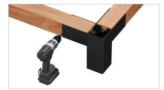
Be sure beam is in contact with bottom of connector and slide beam as far forward as possible. Install screws through holes on sides of connector into beam. (Screws at underside of beams are installed later.)
