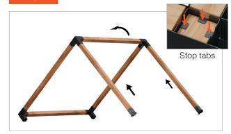
Install post bases onto posts. Lift one side of pergola and insert posts into bottom of corner connectors. Ensure posts are fully inserted (resting against stop tabs).
