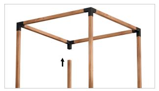
Using a ladder, lift opposite side of pergola and insert posts into other two corner connectors.
