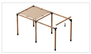
Lower final beam into position between corner connectors. Ensure beam is slotted fully into place, then install screws through remaining holes of corner connectors into beam.
