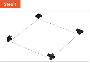
Arrange two (2) corner connectors and two (2) middle-T connectors in a square. To avoid scratching finish, set parts on cardboard or other soft material.
