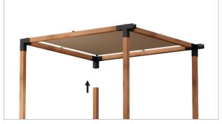
Using a ladder, lift opposite side of pergola and insert posts into other two corner connectors.
