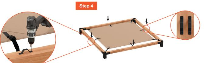
Position remainder of brackets in marked locations and install screws.
