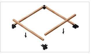
Place beams into connector slots as shown. **Tip:** If a beam's fit is too tight on one of its faces, try rotating it 90°.
