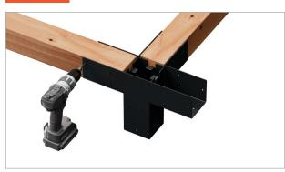
Be sure beam is in contact with bottom of connector and slide beam as far forward as possible. Install screws through holes on sides of connector into beam. (Screws at underside of beams are installed later.)
