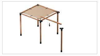
Connect post bases and corner connectors to remaining two (2) posts with only one (1) screw each initially (other screws to be added later). Lift one post into position as shown and place beam between middle-T connector and newly raised post.
