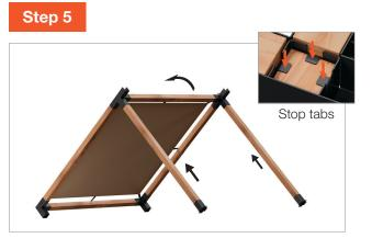
Install post bases onto four (4) posts. Lift one side of pergola and insert posts into bottom of corner connectors. Ensure posts are fully inserted (resting against stop tabs).
