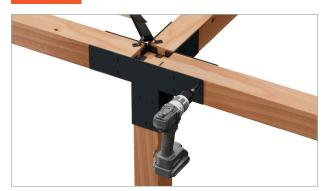
Ensure beam is placed as far as possible into connector. Install screws into remaining holes of middle-T connector. Install screws through remaining corner connector holes to secure beam and post.
