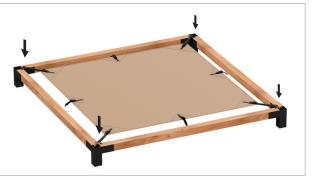
Attach straps of sunshade through brackets installed at each corner. Pull straps to tighten until gap is even on all sides. Do not excessively tighten.
