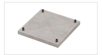
Measure the layout and place post bases in their required position.
