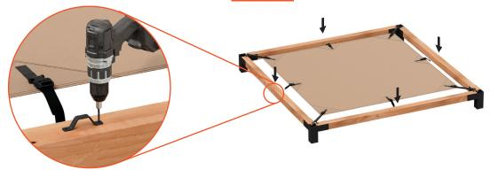
Position remainder of brackets in marked locations and install screws.
