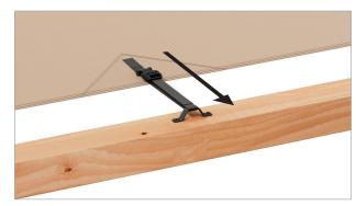
Attach remainder of sunshade straps to brackets. Then pull all straps to tighten until sunshade is snug and gap is even on all sides. Do not excessively tighten.
