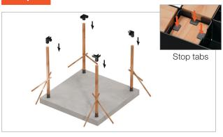
Place corner connectors onto each post and install screws. Ensure post is fully inserted into connectors (resting against stop tabs).
