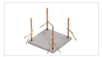
Insert posts into each base. Plumb each post and install temporary bracing. After posts are plumb, install all screws into post bases.
