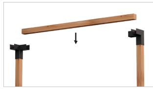
With ladders in place, lift and place a beam into slots of corner connectors. Ensure beam is placed as far as possible into each connector.
