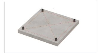
Measure the layout and place post bases in their required position.
