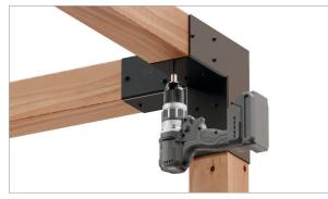
Install all screws into connector on each end of beam. Repeat Steps 5 and 6 for remainder of beams. Remove temporary bracing.
