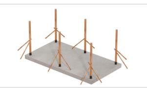
Insert posts into each base. Plumb each post and install temporary bracing. After posts are plumb, install all screws to post bases.
