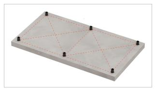
Measure the layout and place post bases in position. **Tip:** The wood beam length should be the dimension between face of post bases. Check diagonal measurements are equal to verify layout is square.
