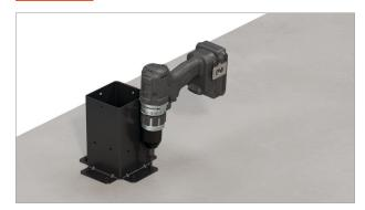
Predrill holes for provided anchors using a <sup>%</sup><sub>6</sub>" concrete drill bit. Install provided screw anchors to secure pergola to concrete.
