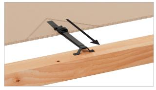
Attach all sunshade side straps to brackets (do not tighten completely until all straps are attached).
