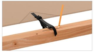
Pull side straps to beam to align bracket and mark bracket locations on all sides.
