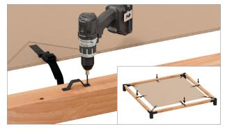
Attach all side brackets in marked locations with included fasteners.
