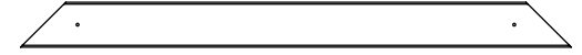
I: Lateral Bracing Support (x8) 2" x 2" x 24" [51mm x 152mm x 610mm]
